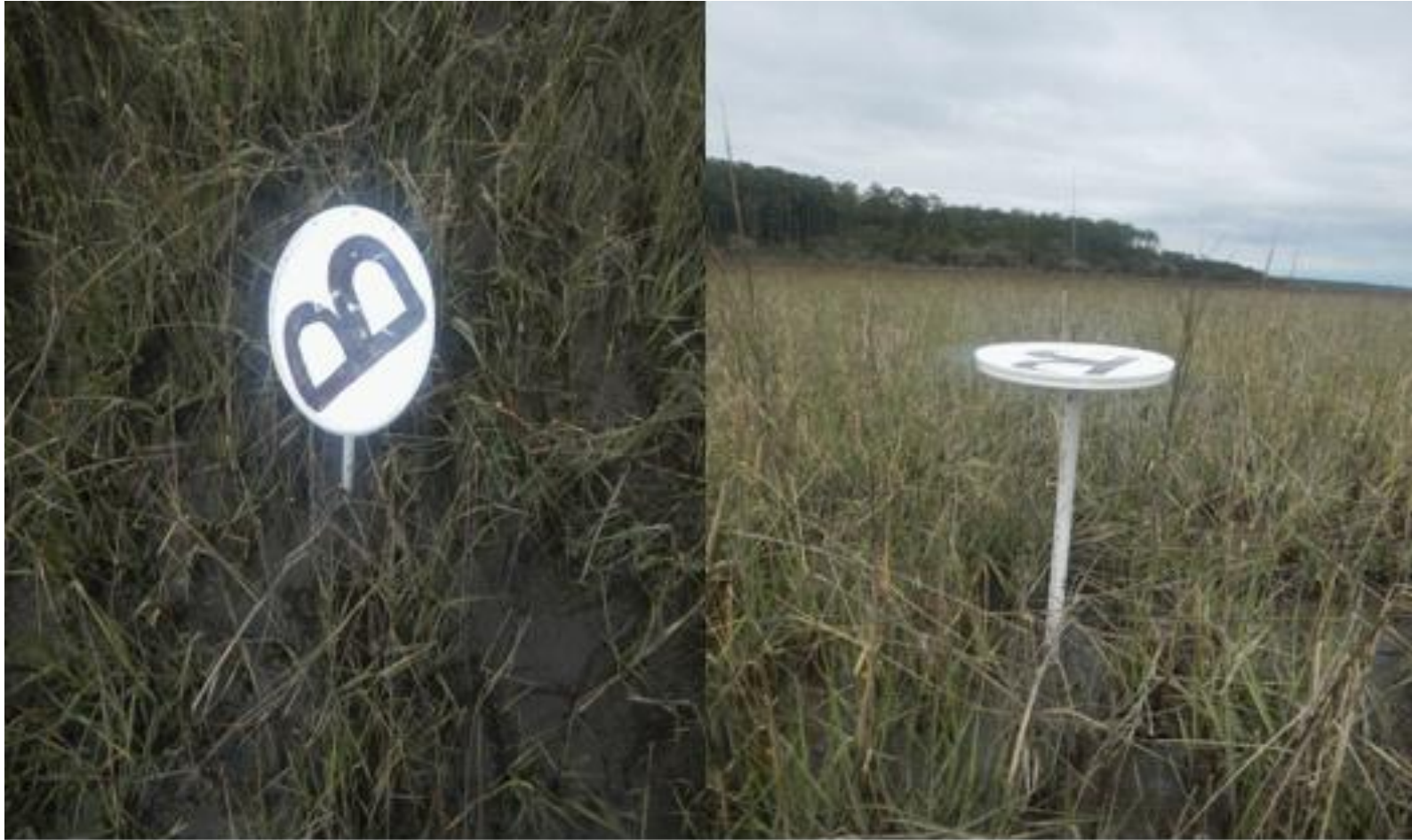
Figure 3.2: Ground control points (GCP) 25 cm diameter bucket lids mounted to PVC pipes.
